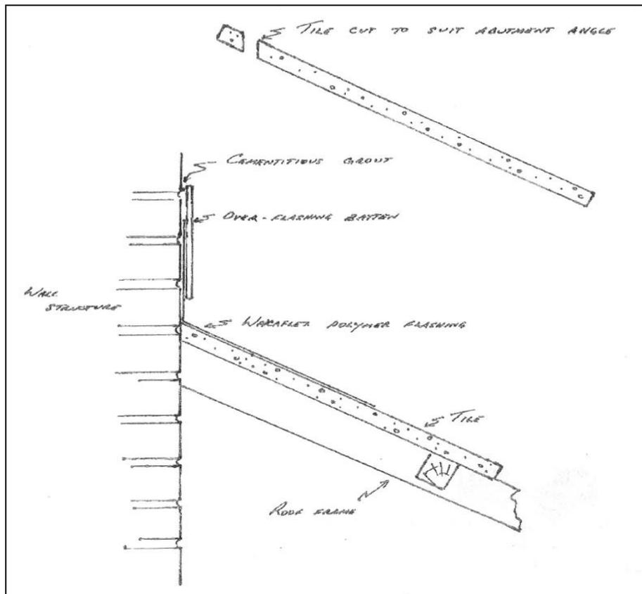
**FIGURE 2.** Cross section of a tile to brick wall system with flashing chased into wall.
